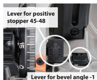
Lever for bevel angle -1
