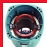
A powder varnish coat on the field coil for protects it from grinding dust
