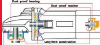
Gears are lubricated by securely sealed grease in gear chamber. Bearings are protected from dust & dirt by labyrinth construction.
