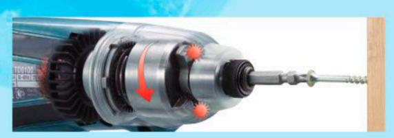
Finally, Hammer delivers enormous impact power onto Anvil, and the tool drives a screw with the high torque which rotational power alone cannot produce.
