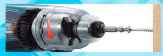
Hammer is now pulled closer to Motor, and finally the protruding portions of Hammer slip under Anvil, resulting in the release of tremendous energy which has been stored in Compression spring. And the released energy powerfully pushes and rotates Hammer.
